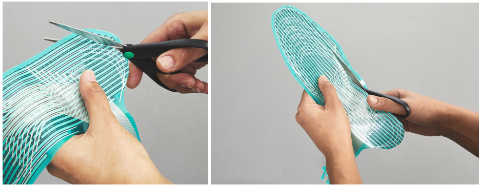
Figure 54 - Trimming the sensors
