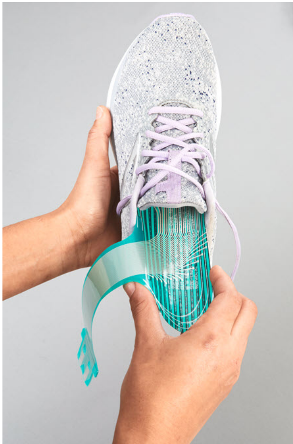
Figure 55 - Fitting a sensor inside a shoe
