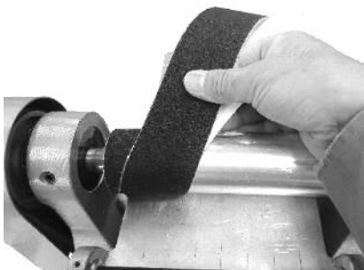
Paste from the edge without gap.
