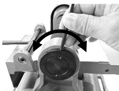
Fine adjustment of height
