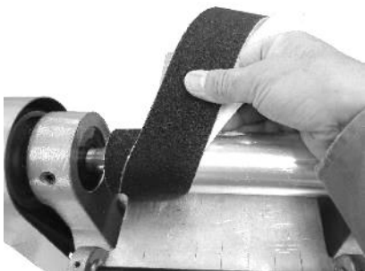
Paste from the edge without gap.
