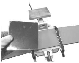
The belt that was removed from the Heat press, Use it after cooling for 1 hour or more.
