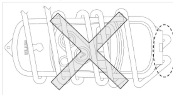
It causes the cable disconnection.
