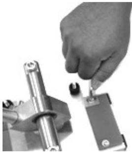
② Change the position of the cutting sheet by sliding it forward or back in the hole on the belt guide.
