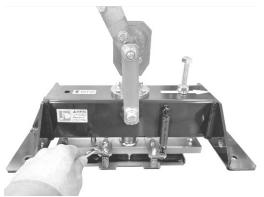
② The nut of the eject plate fixation bolt is loosened.
