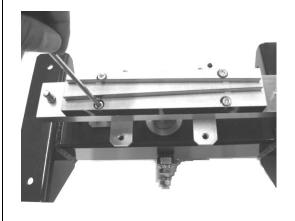
4 Loosen the bolt, and the cutting blade are detached.
