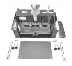
② Reverse the cutting sheet to turn the unused side up and insert it back to the finger puncher.
