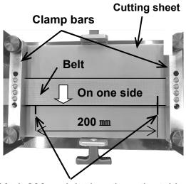
Mark 200 mm joint length on the table. Set both belt ends to same side of the clamp.
