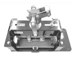
③ Installed the springs, the clamp bars and the bolt.
