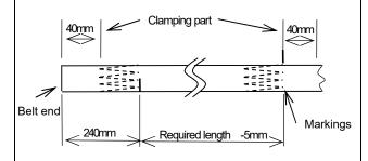
Measure length from finger end (For continuous measuring)
