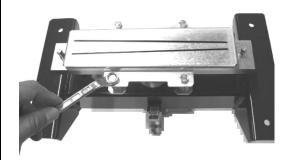
3 Loosen the bolt, and the eject plate are detached.
