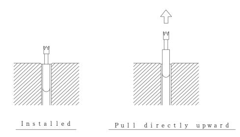
Fig. 14. Tool side spring pin replacement
