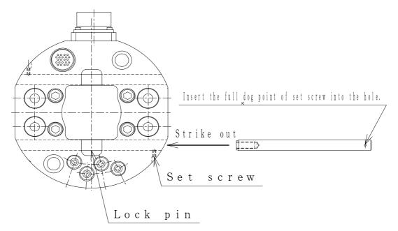
Fig. 19. Lock pin replacement
