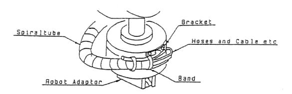
Fig. 5. An example of cable fixing
