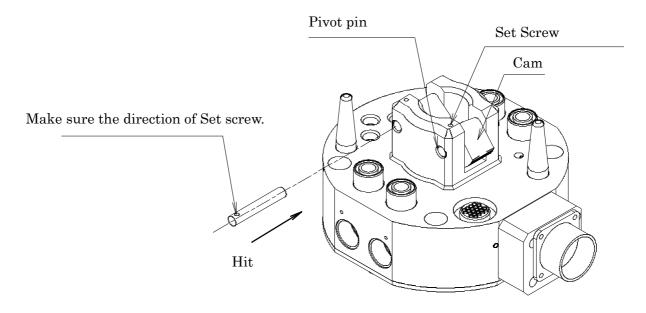
Fig. 20. Pivot pin and cam replacement
