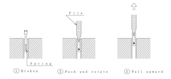
Fig. 15. Pulling out a broken pin
