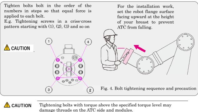
Further, tightening bolts with torque below the specified torque level or failure to use the locking agent may cause bolts to be loosened, leading to module fall off.
