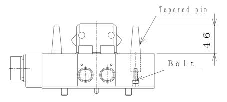
Fig. 17. Tapered pin replacement
