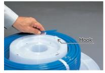
2-3 Fixing inside tubing end and setting reel plate Cover the reel body with a reel plate (A) while inserting the position-adjusted tubing end into an inner-side hole (nearer one of two holes) of the reel plate.
