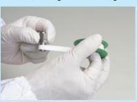
Caution: When reattaching the fitting body, remove the old seal on the thread and bind with new sealing tape. The old sealing tape could contaminate the operating fluid and cause problems.
