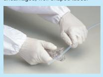
Caution: Do not leave dirt, dents, damage, deformations, burrs, or fluff on the cut surface. Do not cut tubes at a titled angle. The seal of the connection could be damaged, causing leakage.
