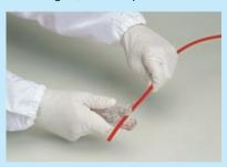
Caution: Do not leave dirt, dents, damage, deformations, burrs, or fluff on the cut surface. Do not cut tubes at a titled angle.
