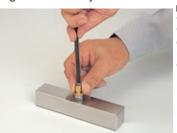
f It is recommended to mark the nut and the fitting body at the hand tightened position in order to check the number of rotations
